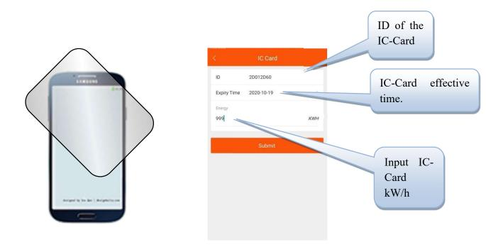
Place the IC card that needs to be added near the NFC module of the phone. After reading the information of IC card, the setting window will pop up. Set the kWh and click ok to add. If there is no response, please change a few more areas to stick, or ask the mobile phone manufacturer to confirm the location of the NFC module.
