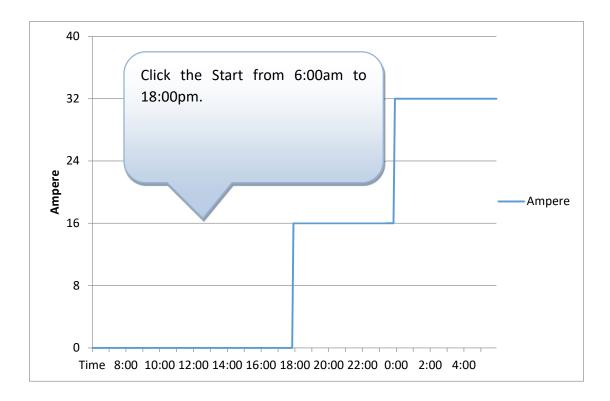
The task activated between start time and end time only. If you click the Start at 4:00AM, the charger will work at default 32A.
