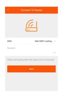
You can set up the charger to connect to a designated router. Press "to connect to the router", and wait for about 10 seconds, then choose router name (SSID) and password. The charger will restart after the setting. Then connect the phone to the router and enter the APP again. You can control the charger within the same network.
